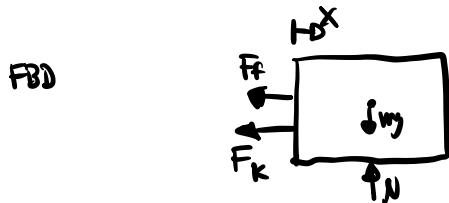
$$-F_f - F_k = m\ddot{x} \Rightarrow m\ddot{x} + \mu mg + Kx = 0$$
